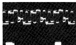
14. Q353 Collector (Y-PCB) 125V, 20 \mu s / Div
