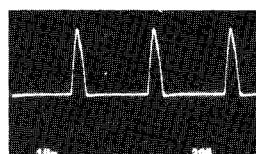
11. FBT Pin 6 (E-PCB) 273V, 20 \mu s / Div
