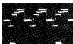
9. E-32 (E-PCB) Green Output From IC601 Pin 16 5.5V, 20 \mu s / Div
