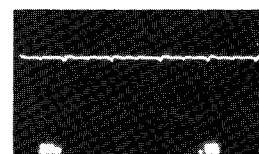
24. IC1101 Pin 12 (E-PCB) Band 1 0.5V, 1 \mu s / Div
