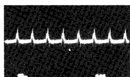
10. FBT Pin 4 (E-PCB) 316V, 50 \mu s / Div
