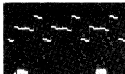
5. IC601 Pin 64 (E-PCB) R - Y In 1.1V, 20 \mu s / Div
