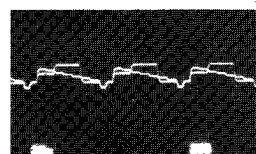
23. IC601 Pin 45 (E-PCB) Vertical Separator 2.0V, 20 \mu s / Div
