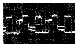
12. Q351 Collector (Y-PCB) 124V, 20 \mu s / Div
