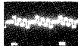
4. IC601 Pin 63 (E-PCB) B - Y In 1.4V, 20 \mu s / Div
