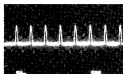
17. Q566 Collector (E-PCB) Horizontal Out 800V, 50 \mu s / Div
